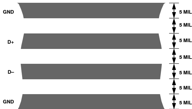
Figure 22. Typical Arrangement of Signal Tracks
